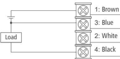
When a current of approx. 125mA/ADC or more is applied, the over current is archived, "Er6" is displayed and the operation stops. Please turn off power supply and check the cause of overload current or lower the current load under 125mA, and then restart the power supply.
