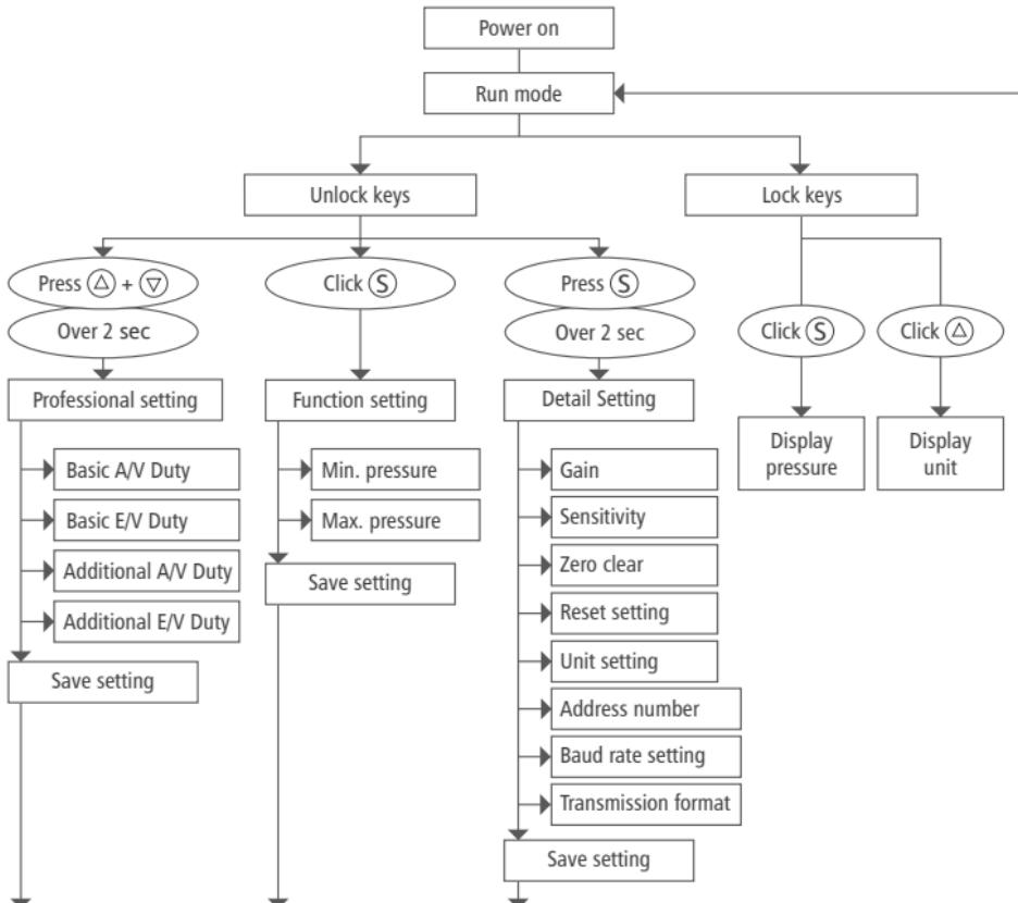
A/V: Air supply solenoid valve ; E/V: Exhaust solenoid valve.
