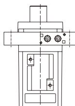
Rod and cylinder are designed for toughness against the large side load. Also suitable for the relatively slowmoving conveyor line with the heavy work carriers.
