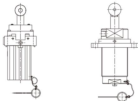
The top rollers with the built-in spring return in touch with the bottom of the work carrier. Automatically returns up to the original position as the work carrier pass by, and immediately works as a stopper for the next work carrier. Therefore the timing carriers does not need to be taken.
